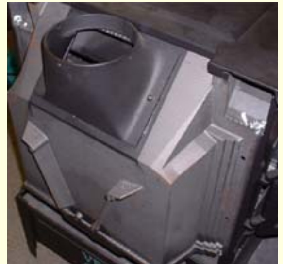
Rear of stove with shroud removed
