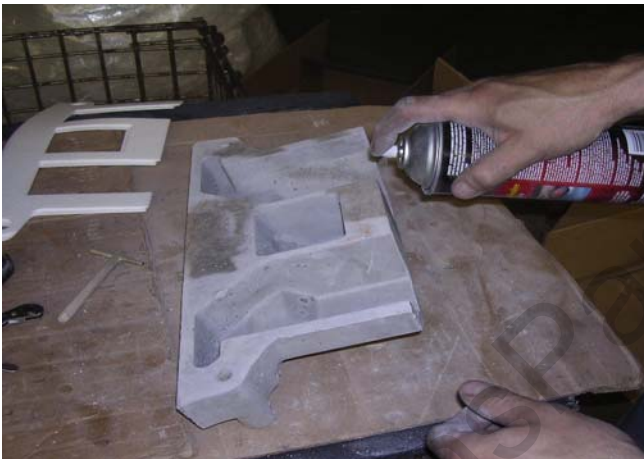
FIG. 36 Shoe Showing Spray Adhesive:
