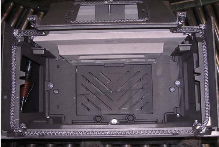
FIG. 38 Inner Top Seal Wrapped Around Sides, Back & Front: Small & Medium 6' x \frac{3}{8} " Fiberglass 1203589
