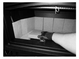
Install the igniter firebrick as shown below. The igniter firebrick has a special hole drilled in it that the igniter will penetrate. Replace the 2 removed floor firebricks.
