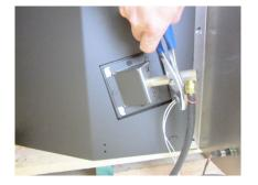
Connect the igniter wires. Orientation of the wires does not matter. Wrap the wires around the compressor hose.
