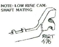
All moving grate pieces have identical mating with the slotted support bracket.
