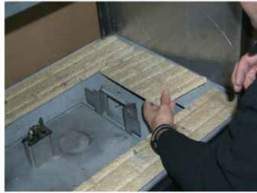
Remove Left & Right Side Base Brick Panels
