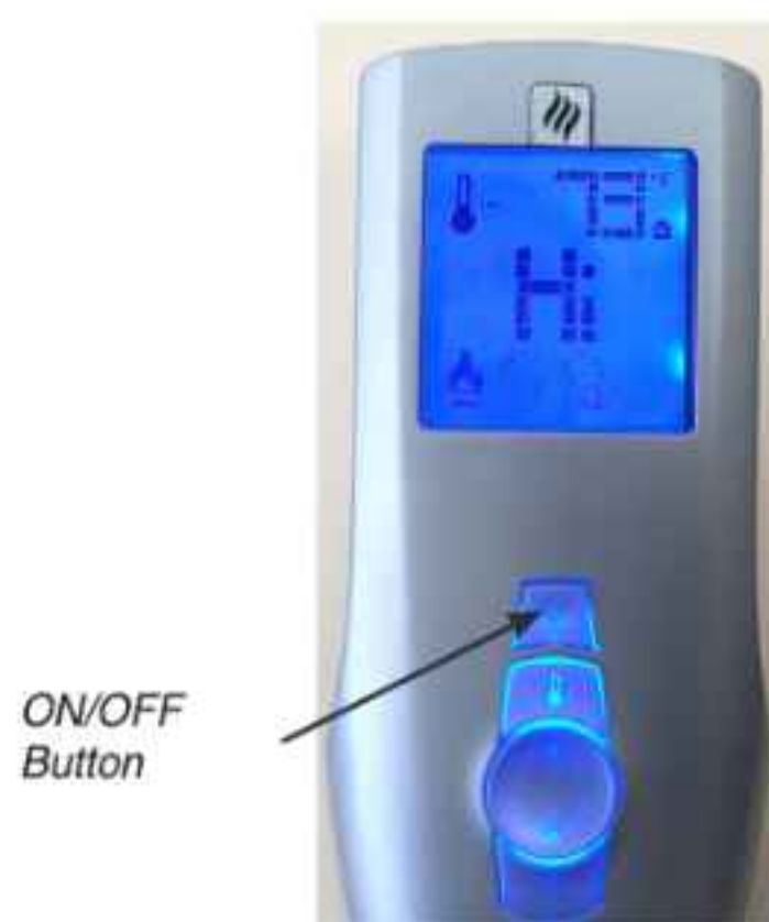
Diagram 1 Remote shown in Manual Mode on Hi
