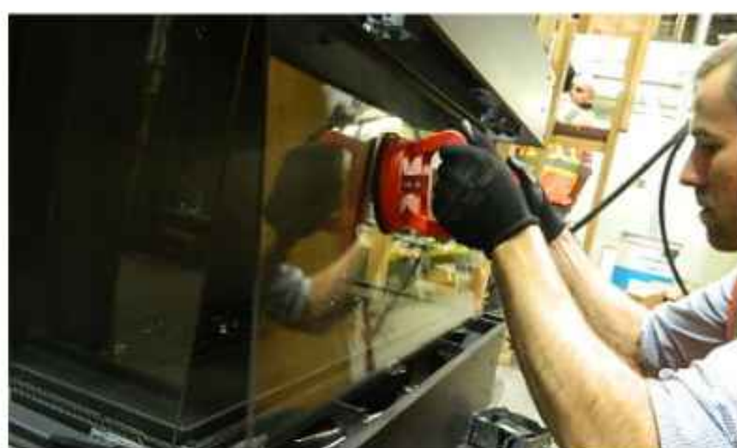
Handle front panel with supplied vacuum clamps
