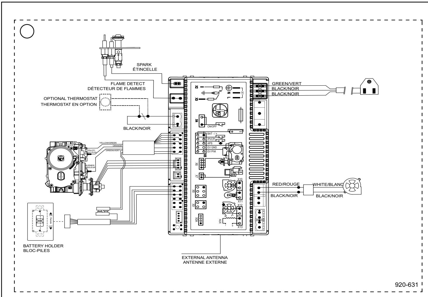
**CAUTION: Label all wires prior to disconnection when servicing controls. Wiring errors can cause improper and dangerous operation.**
