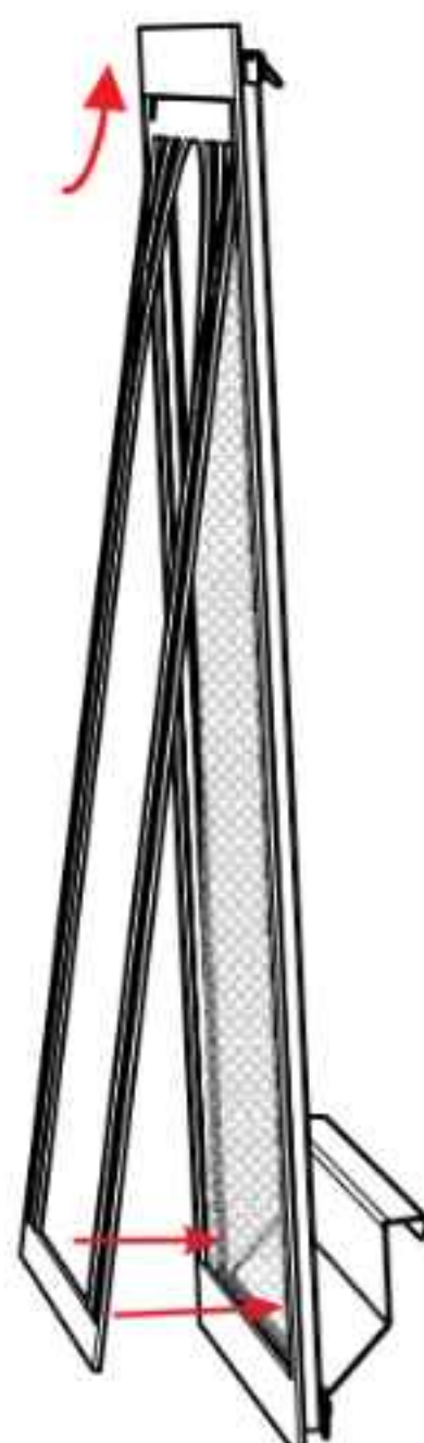
Line up Inlay—Push studs on Inlay through screen
