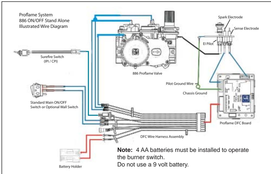
**IMPORTANT:** If the optional remote control is used, the AA batteries normally installed into the battery holder must be removed. The AA batteries in the receiver now operate the unit. Having AA batteries in both the battery holder and receiver will damage the gas valve.
