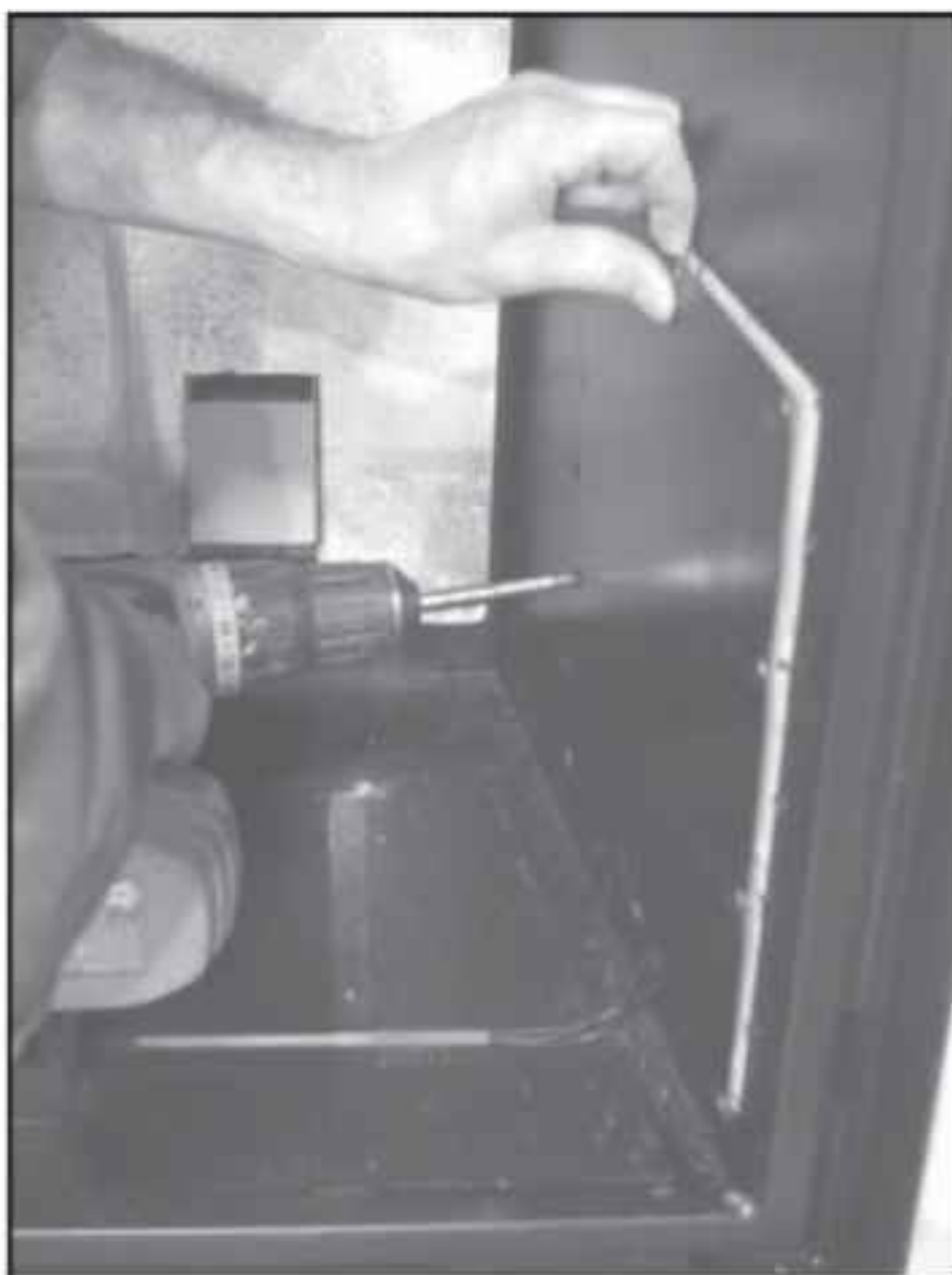
Figure 13: Removing Access Cover.
