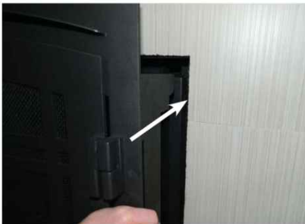
Figure 98: Line up Tabs with slot on Unit
