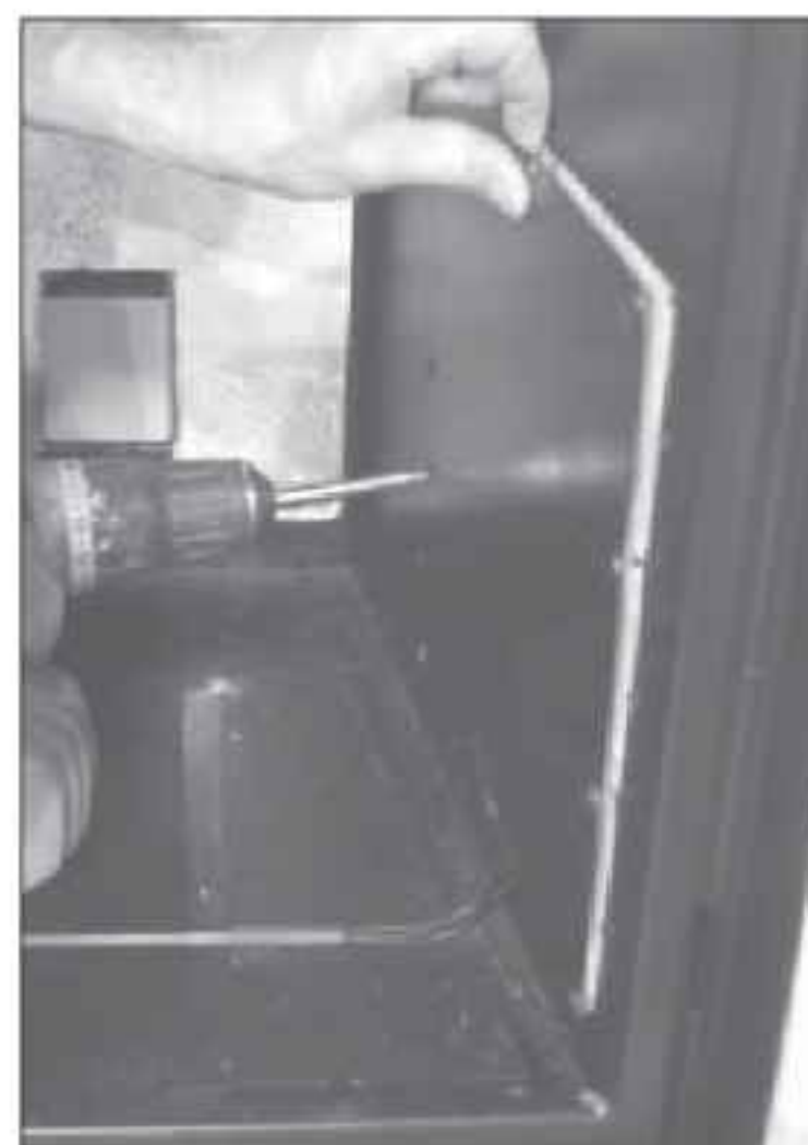
Figure 57: Removing Access Cover.
