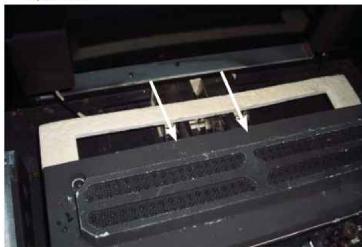
Figure 65: Move Burner away from Mixing Tubes
