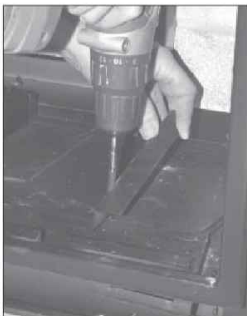
Figure 56: Removing the Right Burner Support.
