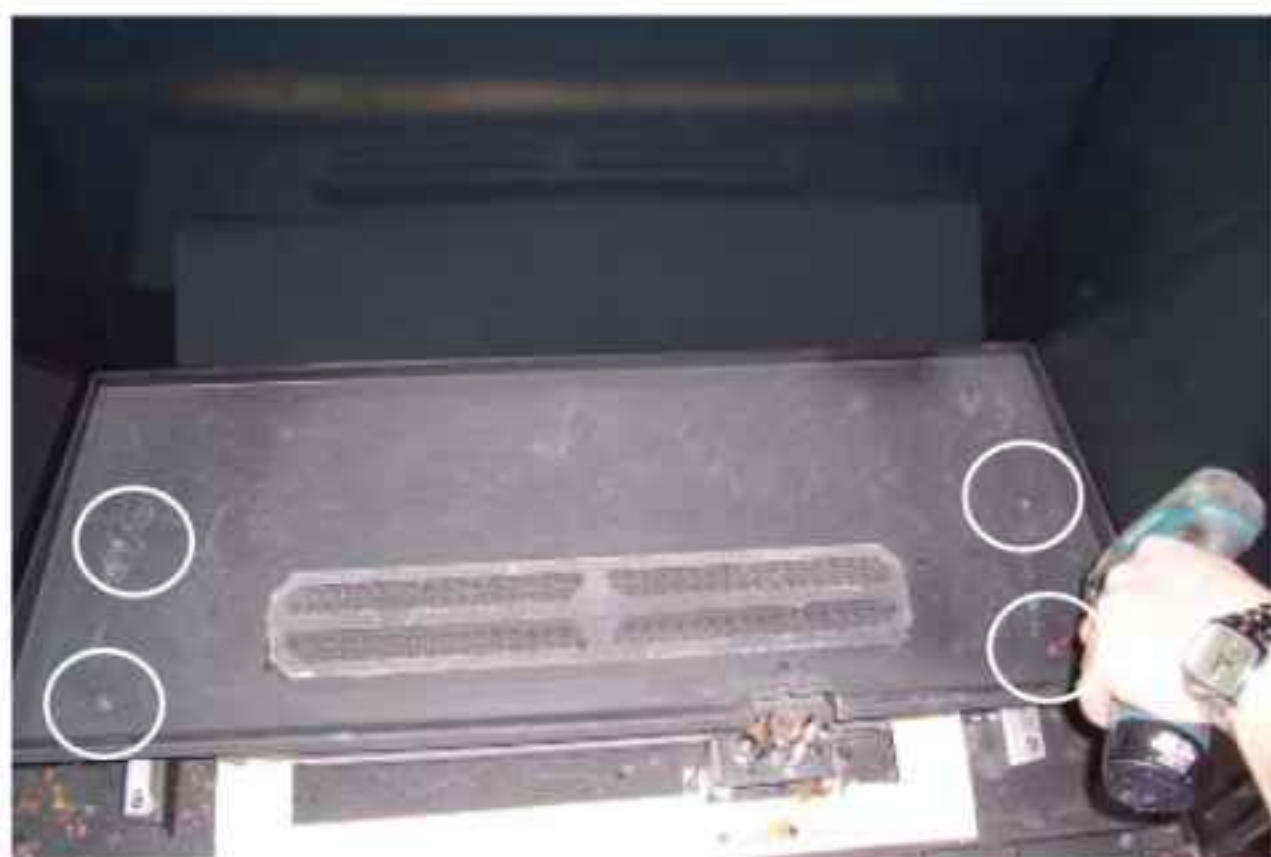
Figure 64: Burner Screw Locations
