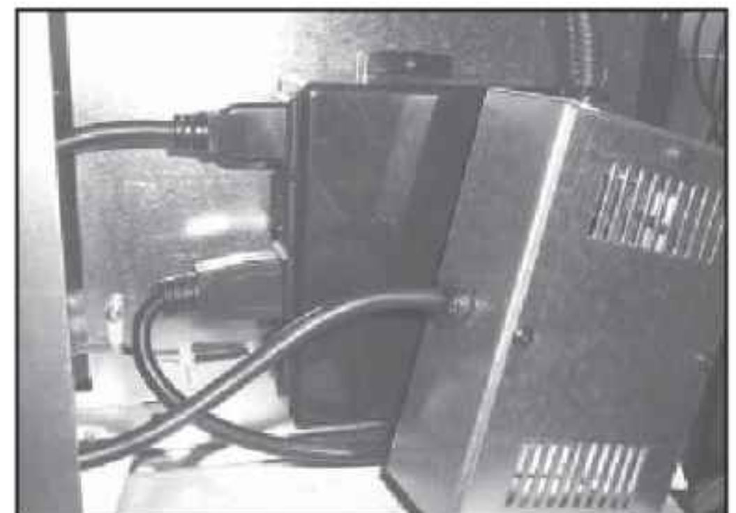
Figure 17: Plugging PVK into Electric Box.
