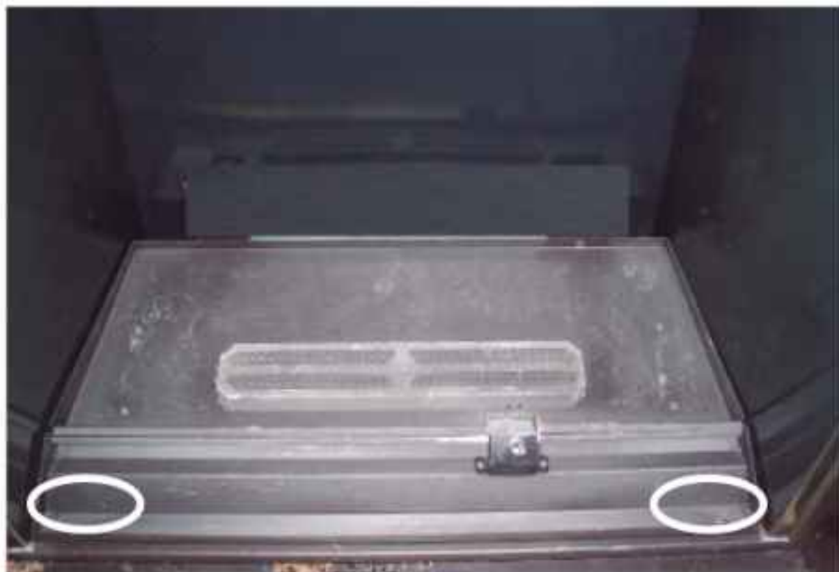
Figure 61: Front Panel Screw Locations
