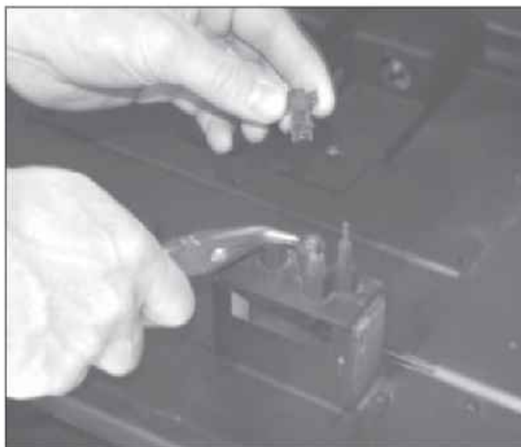
Figure 52: Removing the hood.
