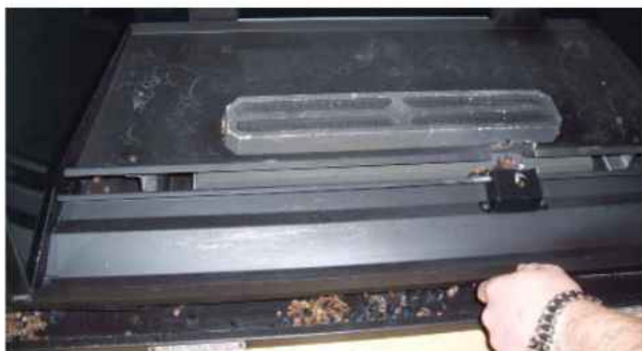
Figure 63: Lift Out Front Panel
