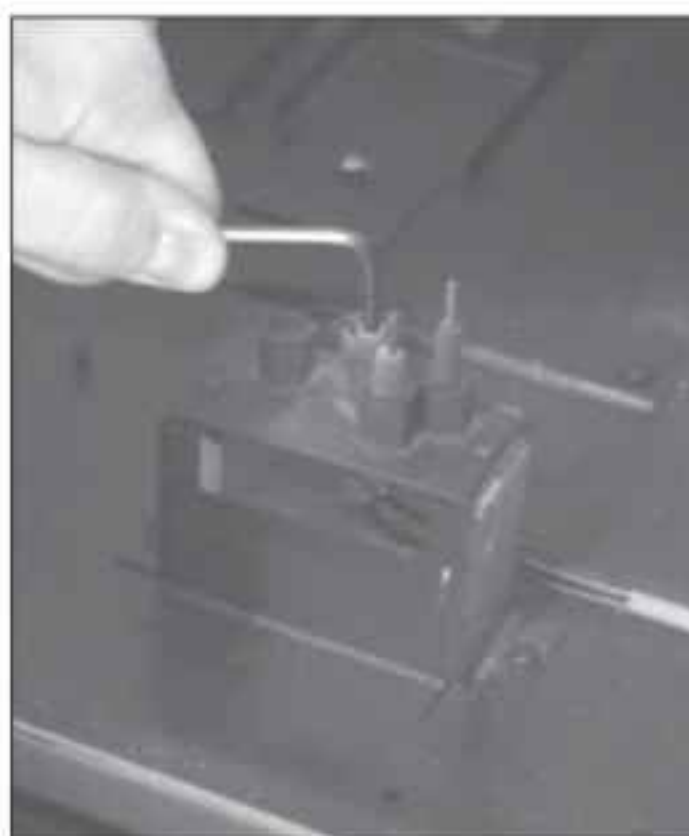
Figure 53: Removing the Pilot Orifice.
