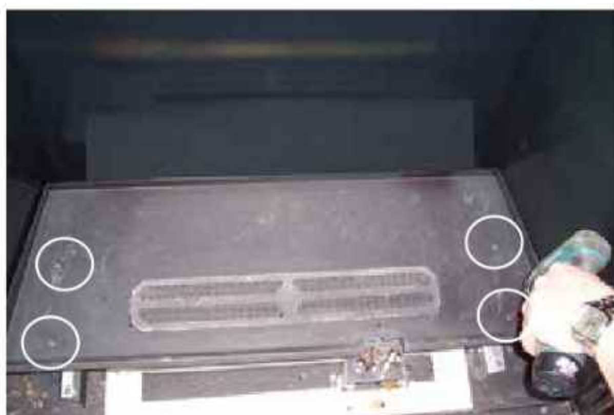
Figure 64: Burner Screw Locations
