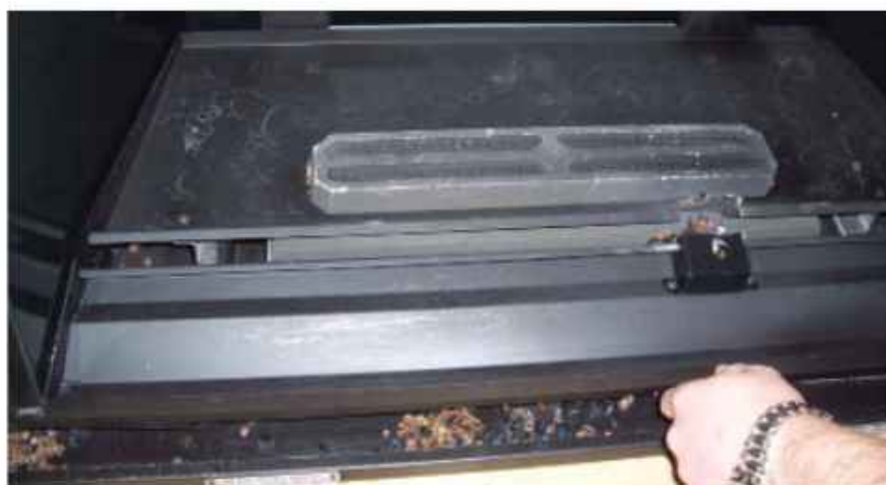
Figure 63: Lift Out Front Panel
