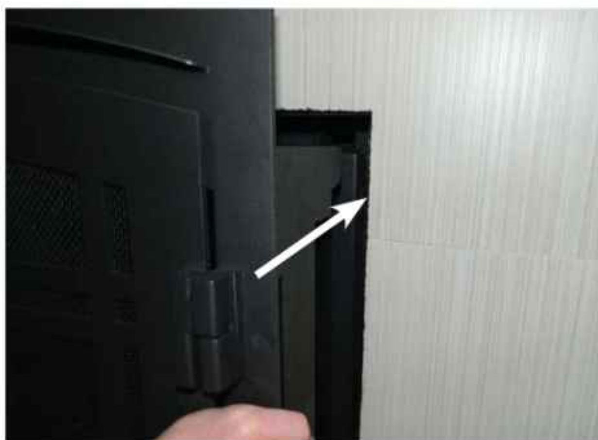
Figure 98: Line up Tabs with slot on Unit
