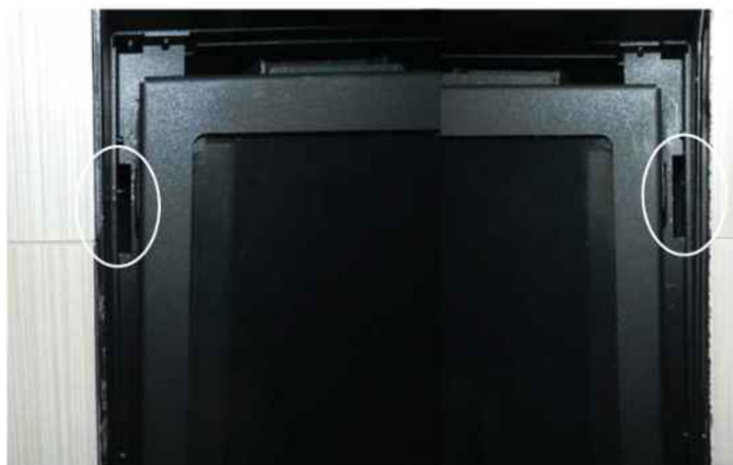
Figure 97: Location on unit to install Full Screen or Screen.
