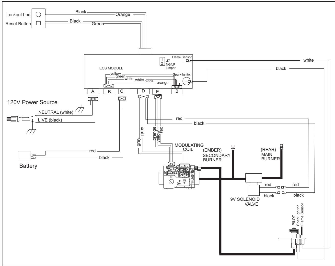
A receptacle is provided on the left hand side of the unit. 120 Volt AC power must be wired to the receptacle and the control module plugged in for the unit to operate fully. The front and rear burners will operate on low, when the unit is running on battery back-up.
