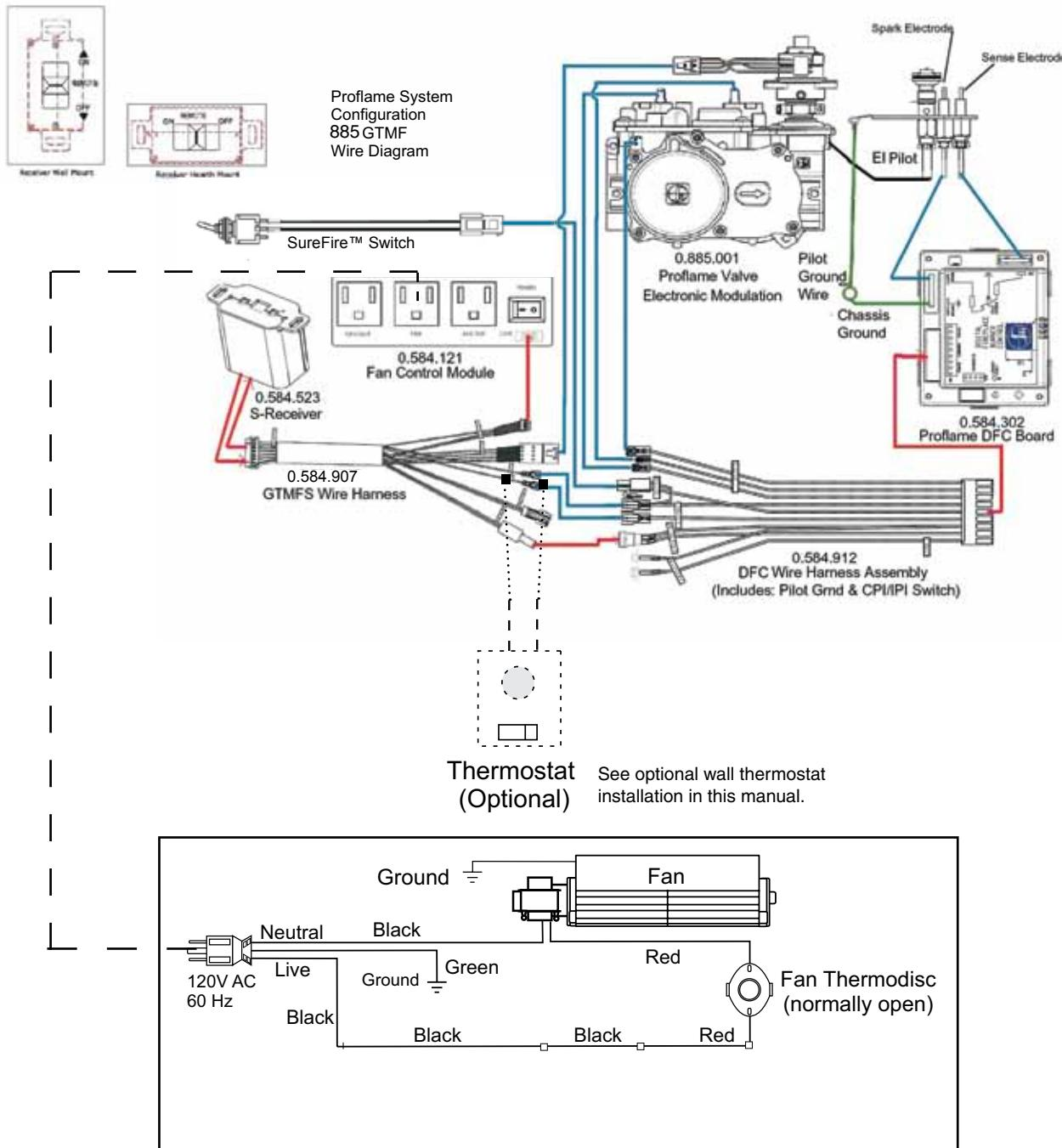
**GTMF REMOTE SYSTEM - IMPORTANT:** The 120V fan control module serves as the power source for this unit. The AA batteries in the receiver only serve as a backup in case 120 volt power is lost within the home.
