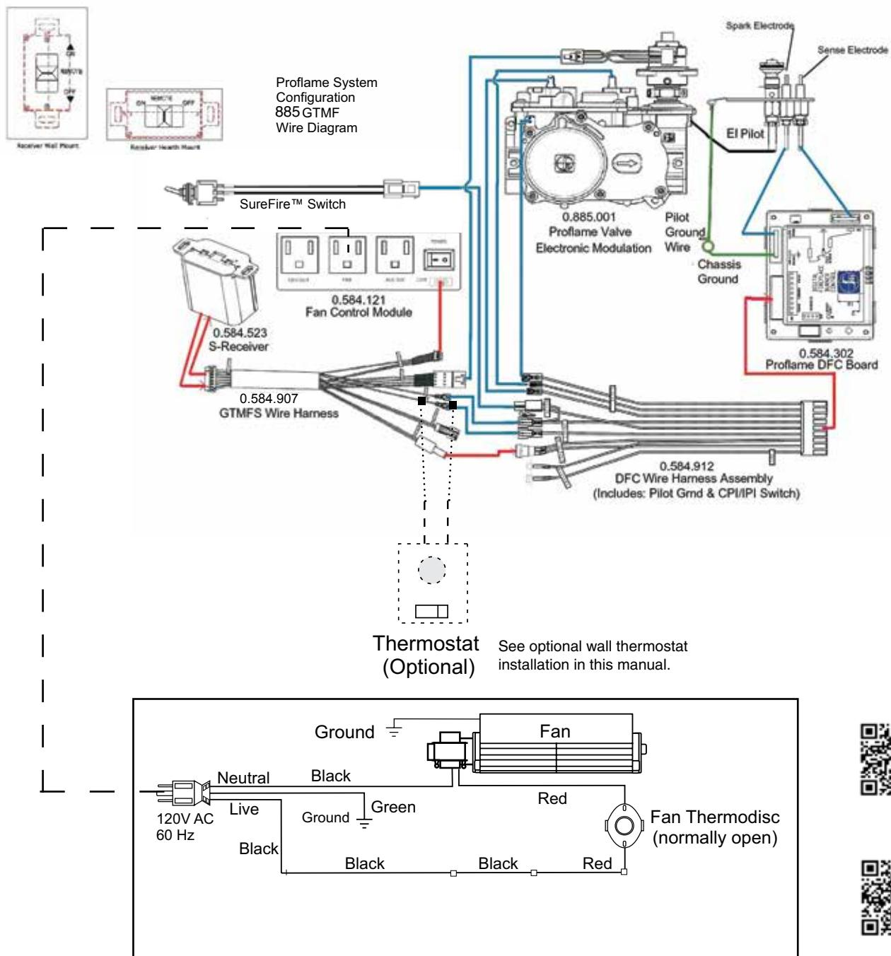
**GTMF REMOTE SYSTEM - IMPORTANT:** The 120V fan control module serves as the power source for this unit. The AA batteries in the receiver only serve as a backup in case 120 volt power is lost within the home.
