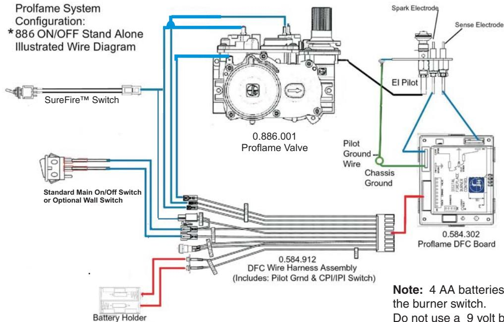
**Note:** 4 AA batteries must be installed to operate the burner switch.
