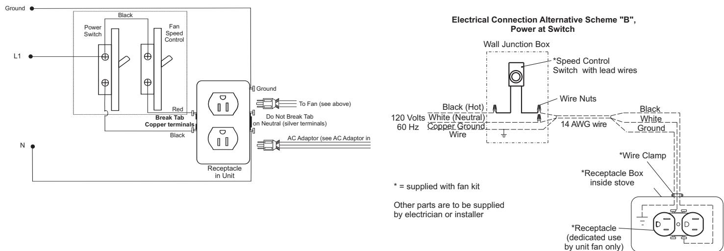
**Caution:** Ensure that the wires do not touch any hot surfaces and are away from sharp edges.
