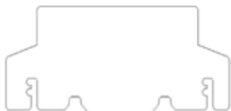
Restrictor plate for Set 1, Set 2 (Part # 761-060F)
