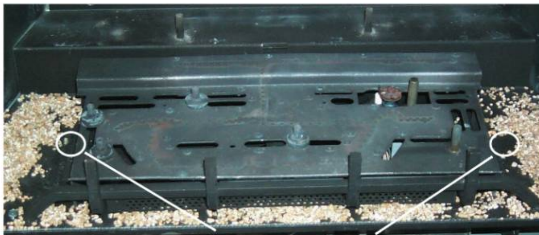
Remove the 2 screws, push Burner Tray to the left, and lift off.
