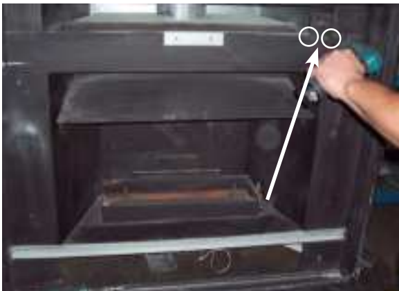
Remove 2 screws - remove Thermodisc Bracket
