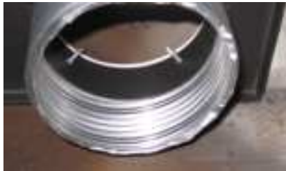
Secure top plate to firebox w/4 screws.
