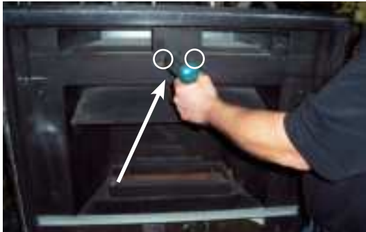
Remove 2 screws - remove Top Bracket
