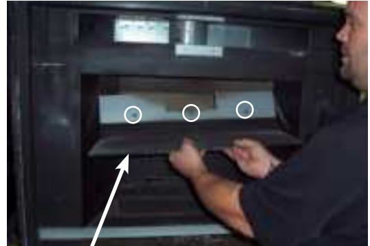
Remove 3 bolts and nuts to remove heat deflector.
