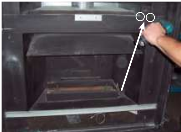
Remove 2 screws - remove Thermodisc Bracket
