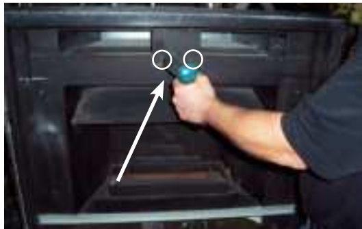
Remove 2 screws - remove Top Bracket
