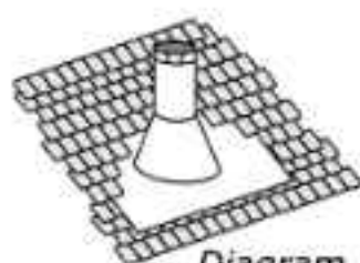
Diagram 1 - The upper half of the flashing is installed under the roofing material and not nailed down until the chimney is installed. This allows for small adjustments.
