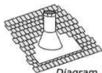
Diagram 1 - The upper half of the flashing is installed under the roofing material and not nailed down until the chimney is installed. This allows for small adjustments.
