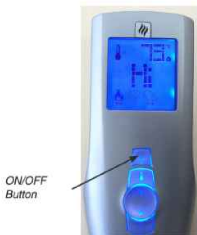
Diagram 1 Remote shown in Manual Mode on HI
