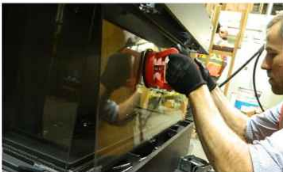
Handle front panel with supplied vacuum clamps
