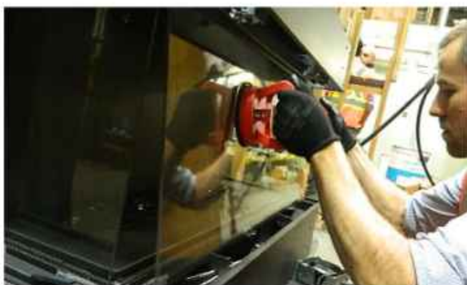
Handle front panel with supplied vacuum clamps
