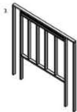
3. Use at least 4 sets of screws to keep the vent flat against framing
