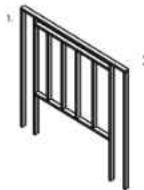
1. Frame opening for vent (See Vent Framing Clearances Page)
