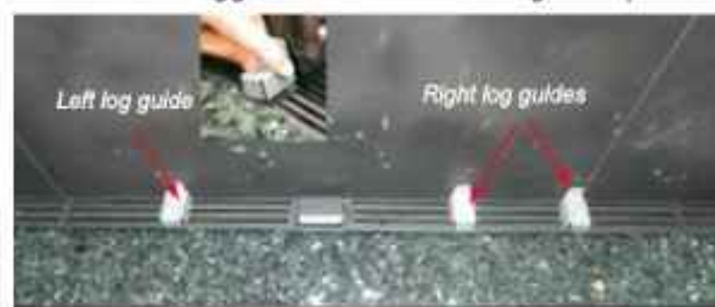
Log guides installed
