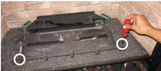
Diagram 1: Remove the left and right screws.
