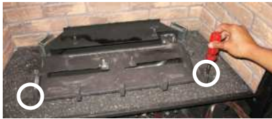
Diagram 1: Remove the left and right screws.
