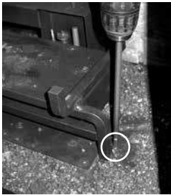
Diagram 1: Remove the left and right screws.
