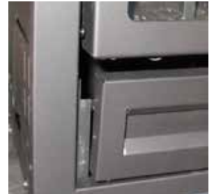
Installation of lower Flush Panel
