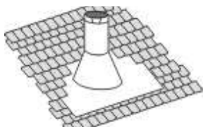
Diagram 1: The upper half of the flashing is installed under the roofing material and not nailed down until the chimney is installed. This allows for small adjustments.
