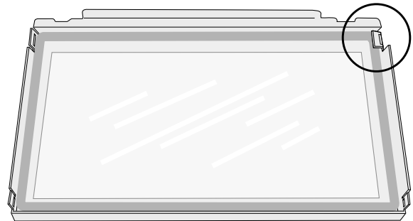
Figure 45. Bend the retainer tabs back enough to release the glass panel.
