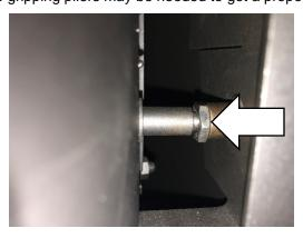
4. Place the bushing, 4700-0915, over the threaded section of the shaft. Install so the shoulder of the bushing is facing away from the body of the stove. Adjust the jamb nut so that the shouldered face of the bushing is slightly protruding from the heatshield.
