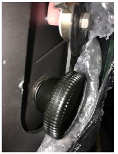
6. Tighten the jamb nut against the back of the bushing. Be sure the knob does not bind against the heatshield. If the knob does bind, loosen the knob and adjust the jamb nut out slightly.
