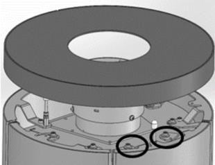
3. Use a ½" wrench to loosen the jamb nut on the back side of the catalyst bypass handle. Spin the jamb nut all the way to the end of the threaded section of the shaft. Remove the catalyst bypass handle from the threaded shaft. Large gripping pliers may be needed to get a proper grip on the knob.
