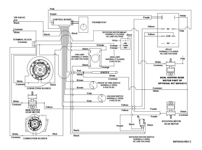
The Electrical Rating of this furnace is: 120 Volt, 60 Hz, 4 AMP. The minimum recommended circuit is 15 Amp. A dedicated circuit for the furnace is recommended.
