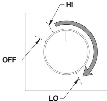
The blower has a variable speed control that can be adjusted in three different positions; either from high (HI) to low (LO) or closed (OFF). Allow the stove to reach operating temperature (approximately one hour) before turning on the blower, since increased airflow from the blower will remove heat and affect the start up combustion efficiency.
