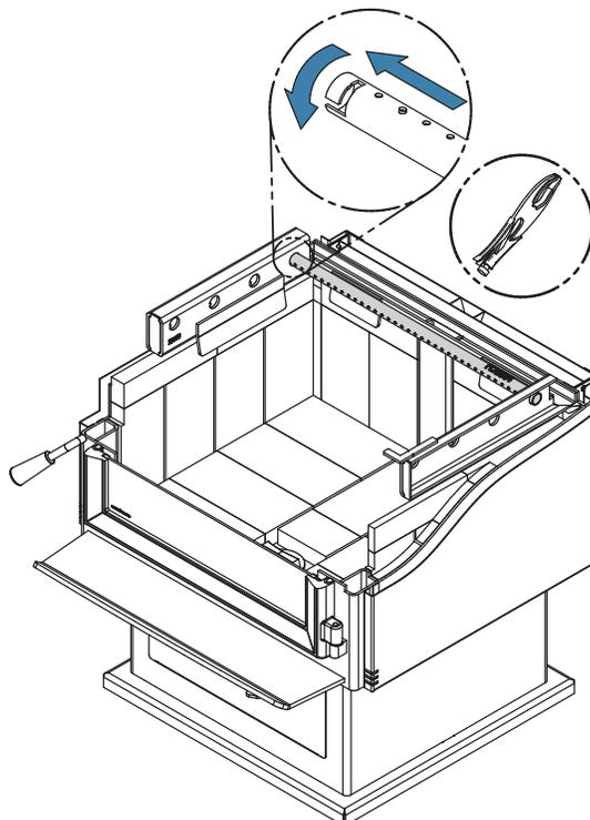
Note that secondary air tubes (A) can be replaced without removing the baffle board (B) and that all tubes are identical.
