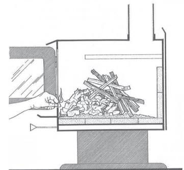
*Do not leave the heater unattended when the door is slightly open. Always close and latch the door after the fire ignites.*
