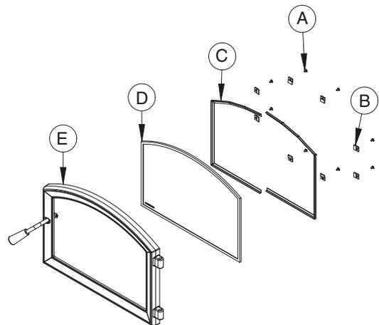
*The two main causes of broken door glass are uneven placement in the door and over-tightening the retaining screws.*
