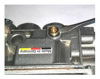
Figure 23 - Low Flow Orifice Removal - O-ring
