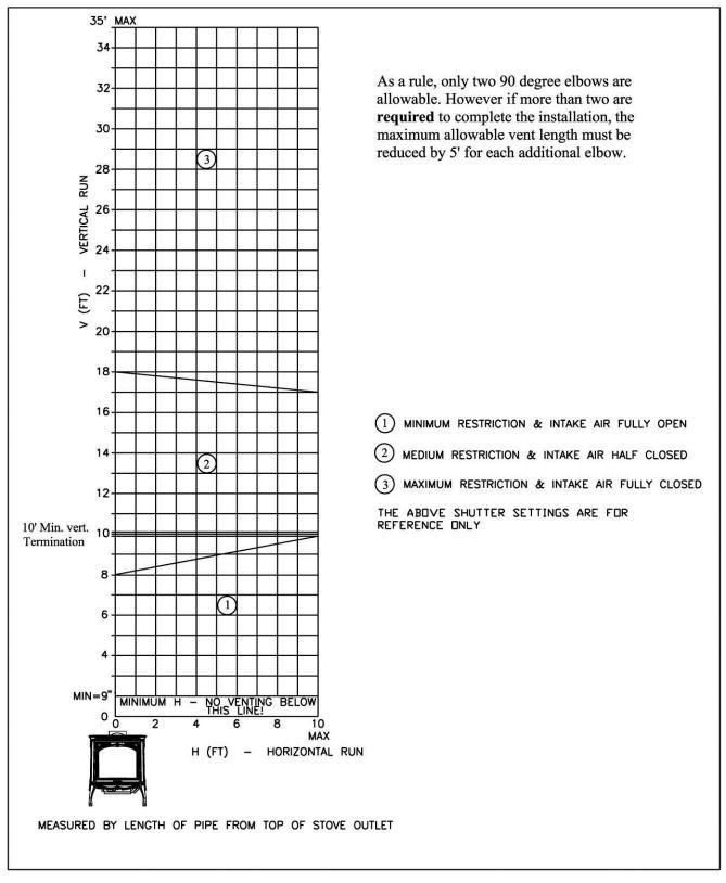
**Figure 13 - Venting Termination Diagram**
