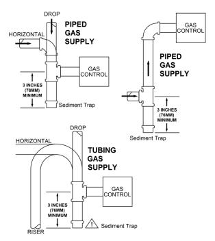
Figure 16 - Sample Gas Supply Sediment Traps
