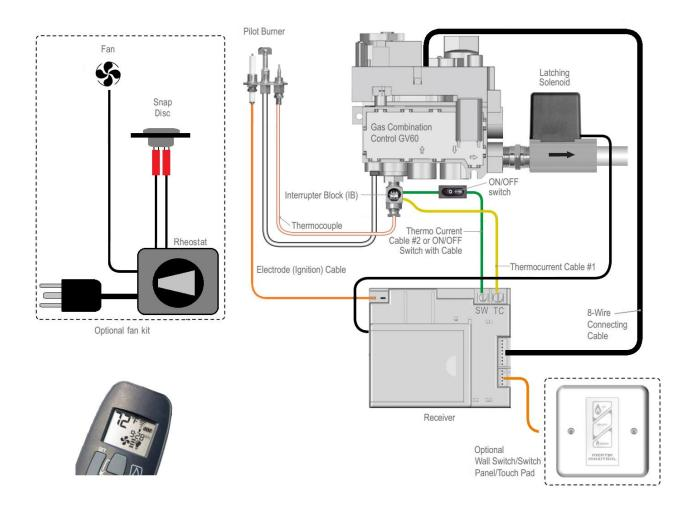
Figure 14 - Stowe 8323 Wiring Diagram
