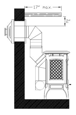
Figure 6 - Horizontal Vent Mantle Clearance
