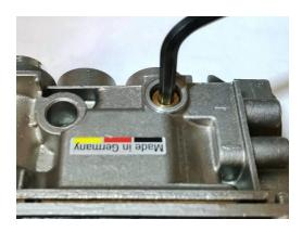
Figure 22 - Low Flow Orifice Removal
