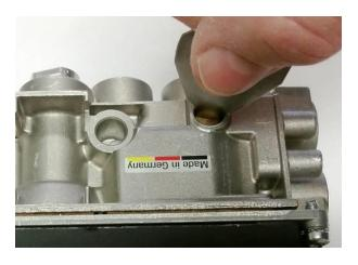
Figure 26 - Tighten LP Low Flow Orifice
