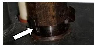
Figure 28 – Loosen Tower and Slide Pilot Gate to Rear of Pilot Tower (LP position)
