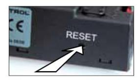
Figure 44 - Receiver Reset Button Location
