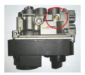
Figure 21 - Low Flow Orifice Location
