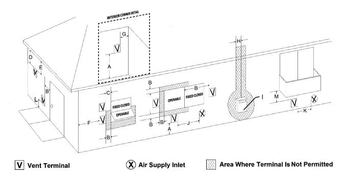
Figure 12 - Acceptable Direct Vent Terminal Vent Cap Locations
