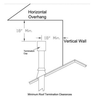
Figure 8 - Termination Cap clearances
