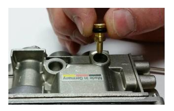
Figure 24 - NG Low Flow Screw Removal
