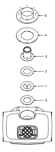
FIGURE 1. GASKET & STOVE ADAPTER INSTALLATION Starter kit pt# 97-60924HB
