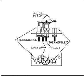
FIGURE 12 PILOT ADJUSTMENT
