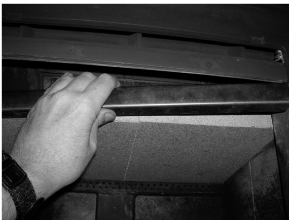
Figure 18 - Removing/Replacing the Baffle for Inspection
