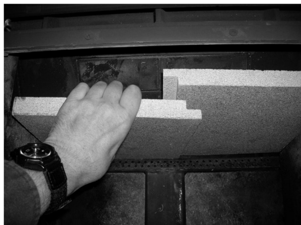
Figure 18 - Removing/Replacing the Baffle for Inspection
