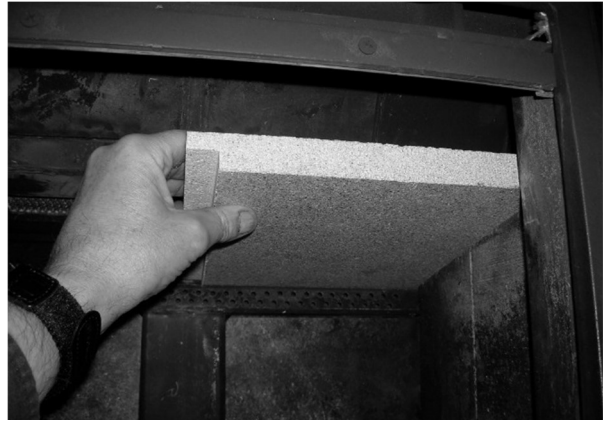
Figure 18 (cont.) - Removing/Replacing the Baffle for Inspection
