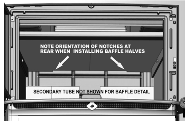
Figure 11 - Baffle Notch Detail
