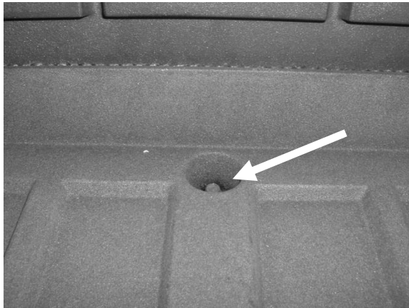
Photo 11 – Rear Leveling Bolt Detail (With Stover lock nut installed - accessed in Firebox)
