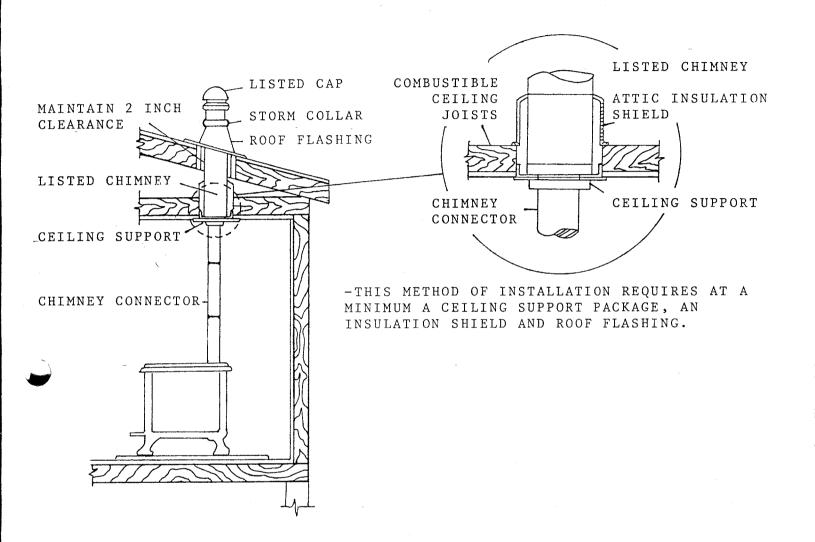
There are basically two methods of metal chimney installation.
