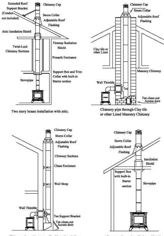
Chimney through outer wall with enclosed chase. Chimney is supported by Tee Support Bracket. One story house installation with attic. Chimney is supported by Ceiling.
