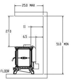
Figure 5: Tribute 8040 Allowable Minimum Alcove Clearances
