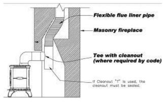
Figure 8: Typical Masonry Fireplace Connection
