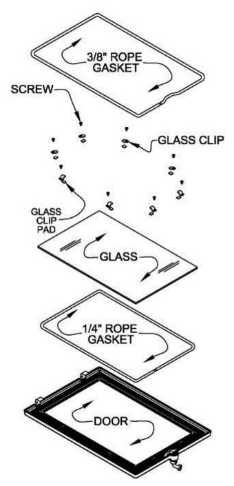
Replace the door glass immediately if broken or chipped. Contact your local dealer for the replacement glass kit PN 90-58405, which is accompanied with instructions and everything needed for the repair. If you replace the glass yourself, wear work gloves and safety glasses. The procedure for glass and glass gasket replacement is as follows:
