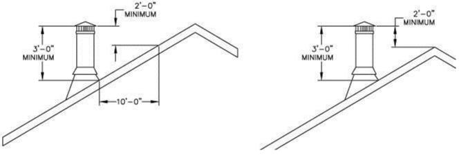
**Figure 9: Chimney Height Requirements**
