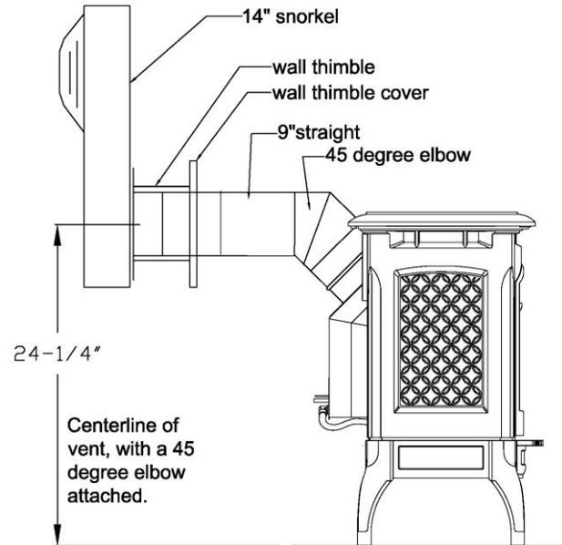
**Figure 17 - Components for a Typical Snorkel Installation**
