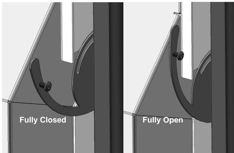
**Figure 20 - Restrictor Adjuster Arm Detail**
