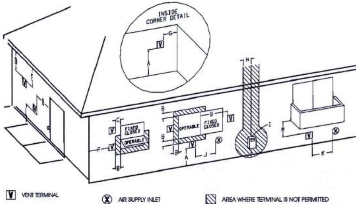
**Figure 16 - Acceptable Direct Vent Terminal Vent Cap Locations**
