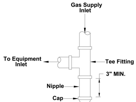
Figure 25 - Sediment Trap (Typical)
