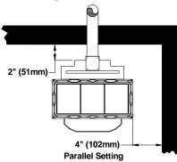
Figure 3: Horizontal Exit Installations
