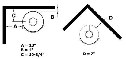
Figure 2 - Clearance to Combustibles
