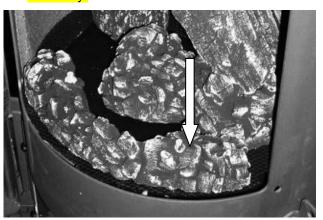
Slide the Right front ember strip next to the Left ember strip. The two fit together to hide the seam.
