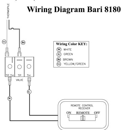
Figure 10: Bari 8180 Wiring Diagram
