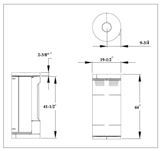
Figure 1: Bari DV Model 8180 Dimensions
