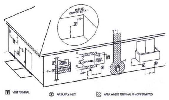
Figure 5: Termination Location & Clearances
