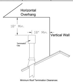
Figure 9: Termination Cap clearances
