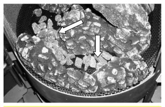
Sprinkle the charcoal embers over the burner ports <u>only</u>. Ensure that you leave the ports open over the pilot and where the main burner ignites.
