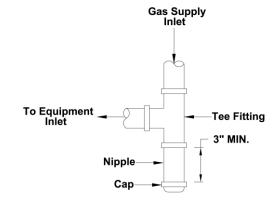
Figure 12: Typical Sediment Trap (required in all installations)
