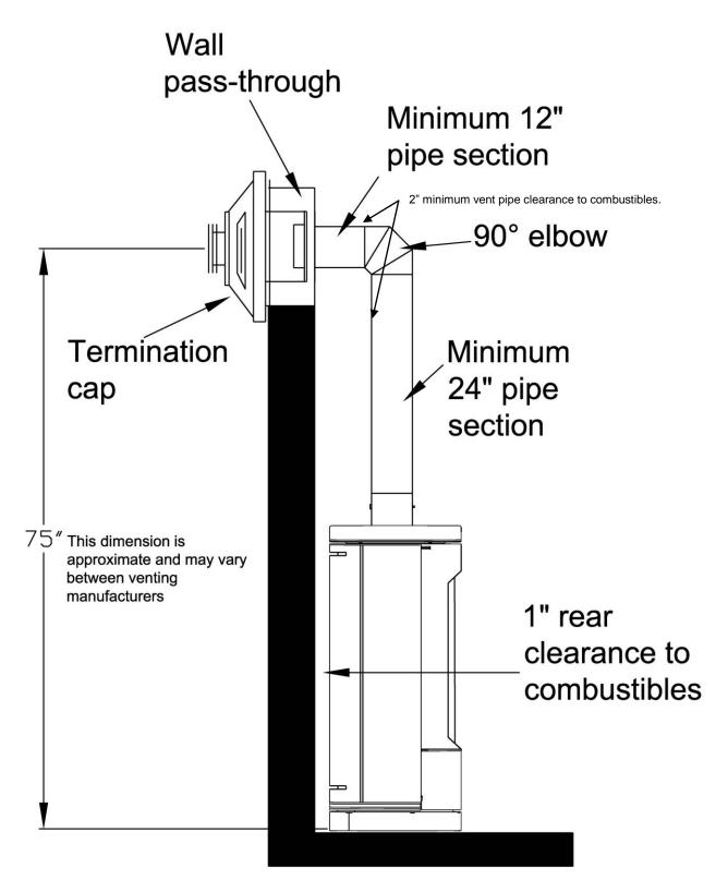
Figure 4: Minimum Vent Configuration and Clearances
