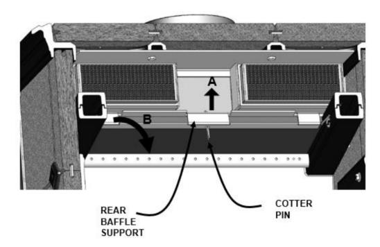
4) Pull rear baffle support (B) outward towards the front of the stove, and remove from firebox. Save for reinstallation. Remove broken rear baffle.
