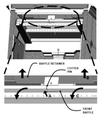
2) Pull the front baffle towards the front of the stove (C), over the front tube, and out of the stove.
