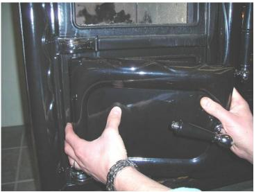
**Photo 4**Remove the ash door in the same way the firebox door was removed.
