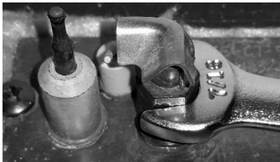
Figure 2 – Loosening Pilot Tower
