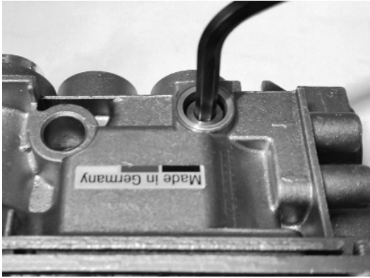
Figure 13 – Loosening Low Pressure Orifice
