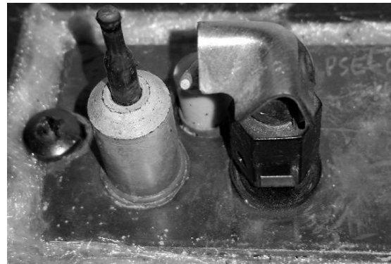
Figure 4 – Correct Pilot Hood Orientation
