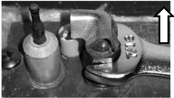
Figure 8 – Loosening Pilot Tower
