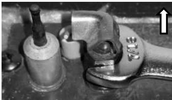
Figure 2 – Loosening Pilot Tower
