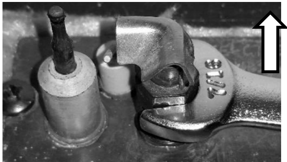
Figure 8 – Loosening Pilot Tower
