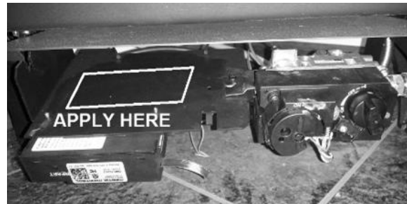
Figure 14 – Rating Plate Conversion Label Location
