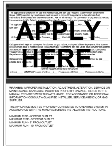
Figure 13 – Rating Plate Conversion Label Location
