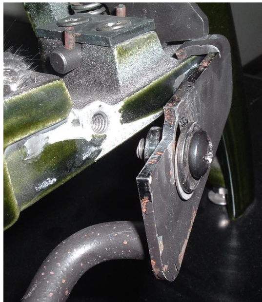
Photo 3: The ash lever pulled away from the top of the ash door. Ash door is open and tilted door for access.
