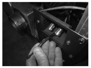
8. Pull out approximately 9" of sensor wire. Use the included wire clamp to secure the sensor wire to the back of the stove as shown below – the end of the sensor should not contact any material (it should be open to air). Use the included lock-tie to secure any excess wire inside the stove.
