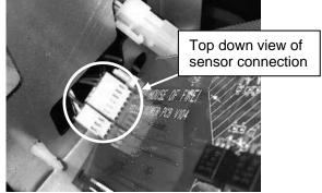
**NOTE:** It is possible to connect the sensor one pin off, causing the inaccurate reading.
