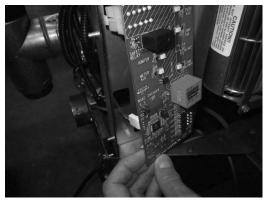
3. Disconnect the harness leading to the user-interface (UI). NOTE: This connection is difficult to remove. You must pull the harness away from the locking tab (to the left).
