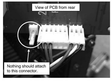
If the connections are correct and the problem persists, perform the voltage test that is explained in detail in the "Testing DC voltage from the Temperature Sensor" section of the "Deerfield/Foxfire Troubleshooting and Service Guide", available in the back office.
